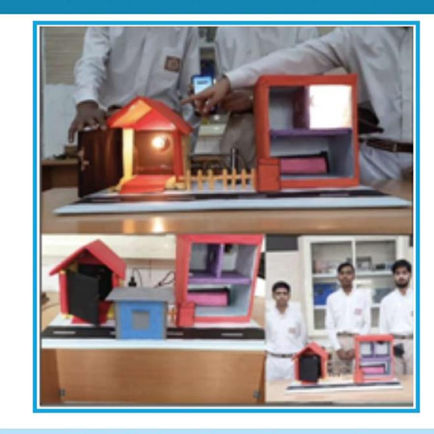
SWITCH OFF the appliance using the smartphone. It's not just controlling the home appliances using the phone but it also protects from a theft attack. Bluetooth app and coding through ARDUINO UNO has been used to develop this model.
