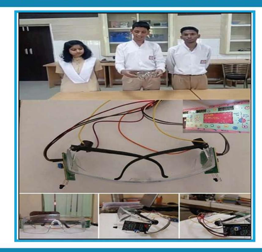
obstacle is below 20 cm (One can change to any desired value). The person wearing specs will get an alert over the buzzer (We have used a melody tone as the alert) attached to the specs and become aware of that obstacle. So, the collision will be prevented.
