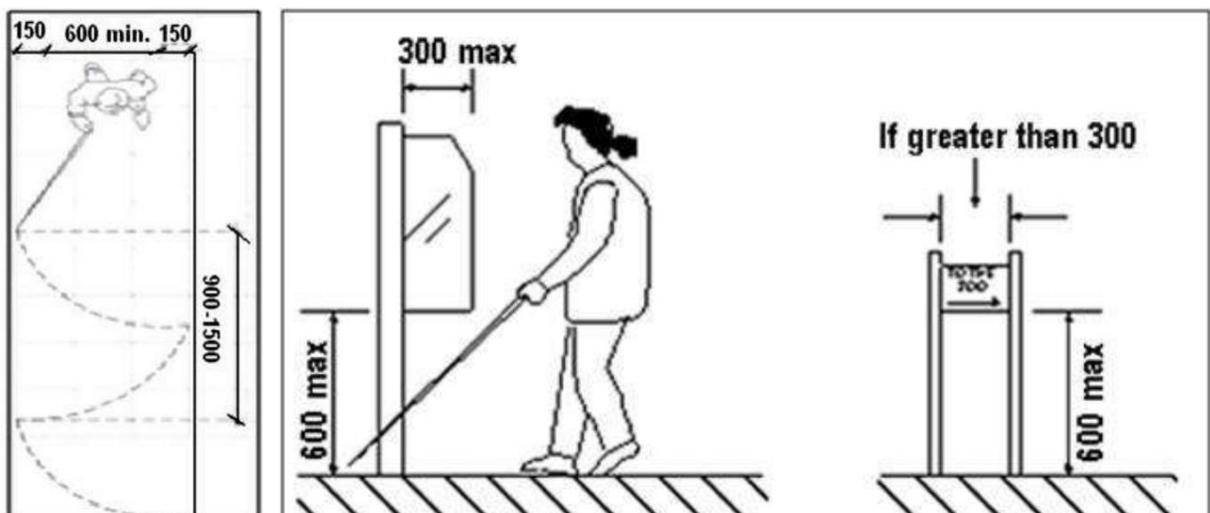
Figure 4.6: Radial range and object detection by the persons with visual impairment
